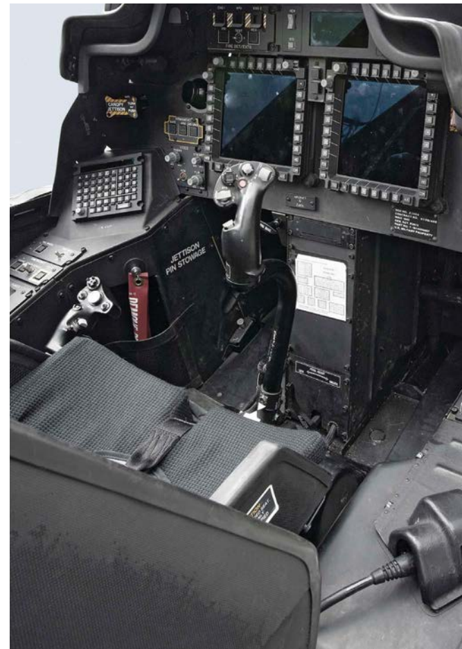
► INSTRUMENT PANELS The pilot sits above and behind the co-pilot/gunner. All the helicopter's systems are displayed in both cockpits and managed using the buttons around the screens.
